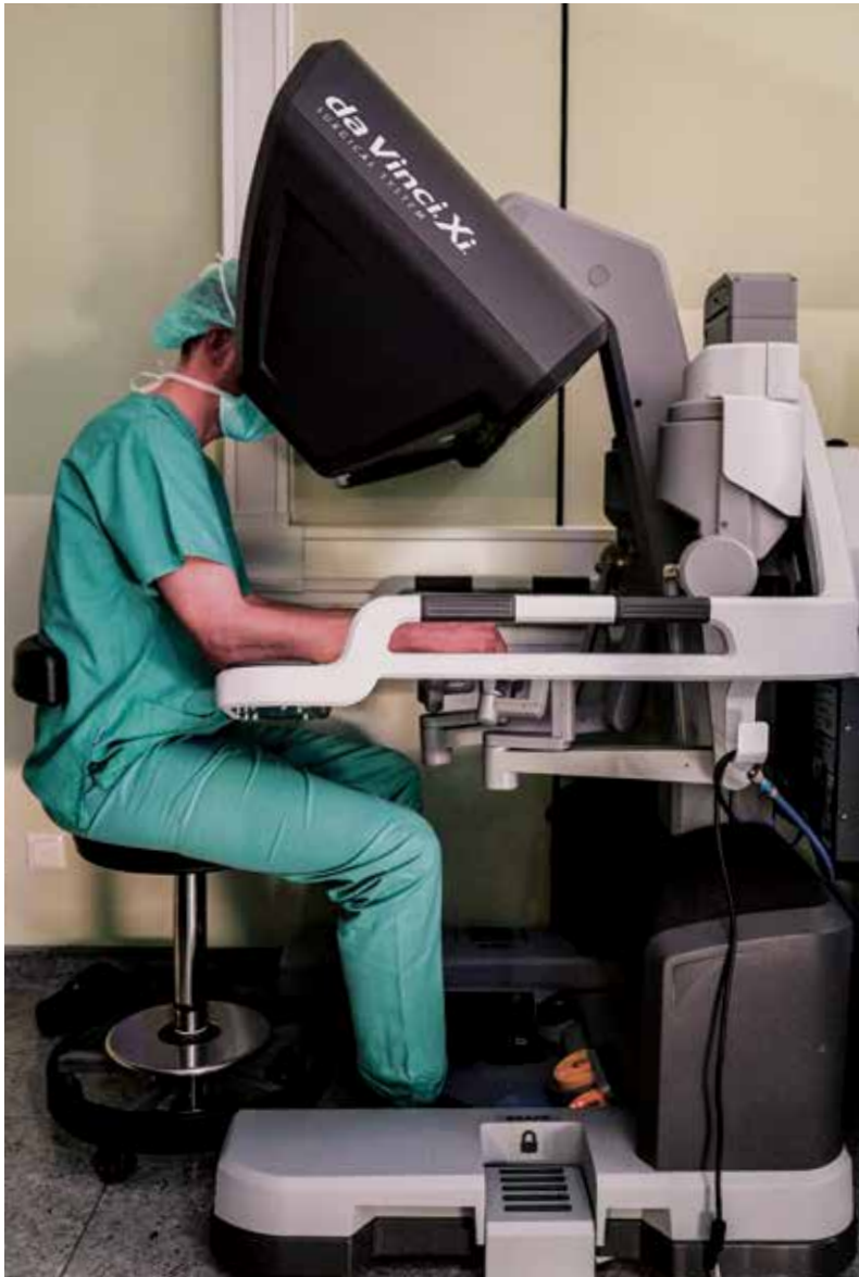
The posture of the surgeon at the console of the Da-Vinci XI
